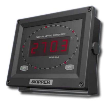
DGR 360 is a digital gyro repeater that displays the Heading Angle in the LED segment display and indicates the Direction of Turn with 30 dual-color surrounding LED's, changing from green to red colour depending on the direction of turn.
